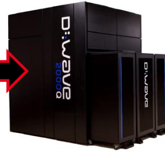
Magnetically shielded enclosure (10 -9 Tesla)
