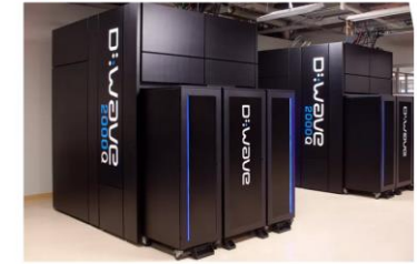
Quantum computing is a very complicated subject branch of computer science that could one day radically change the way our computers function. At the forefront of that field is a Canadian company called D-Wave, which created the world's biggest quantum computing chip last year: with over 2000 qubits (quantum bits) to perform calculations. Now, that chip is finally shipping in a 10-foot tall, $15 million dollar quantum computer called the D-Wave 2000Q , which is a successor to the company's earlier 1000Q, which only had half the number of qubits.
